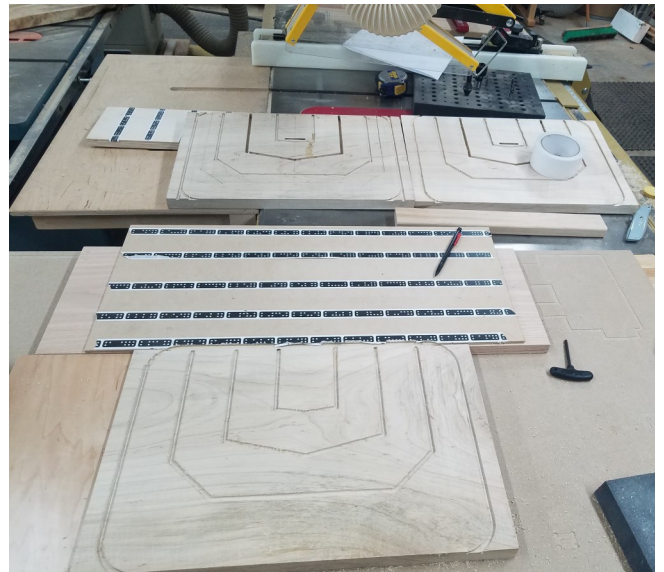
Using the Shaper Origin to layout the contour of the chair seats and profile
