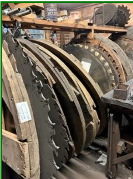
Saw blades ready to be repaired
