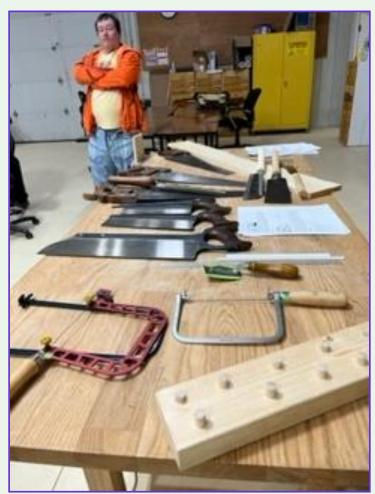
Shawn Jarvis and Tim DuBois brought all sorts of handsaws, including a coping saw, a fret saw, a veneer saw, several back saws, a dovetail saw, and Japanese saws. Members got a chance to saw sample boards with them. The big hit of the evening was Tim DuBois' dovetail saw he has had in a drawer for years, but he's going to start using it now! Many people decided they wanted to buy a Japanese saw as their next purchase.
