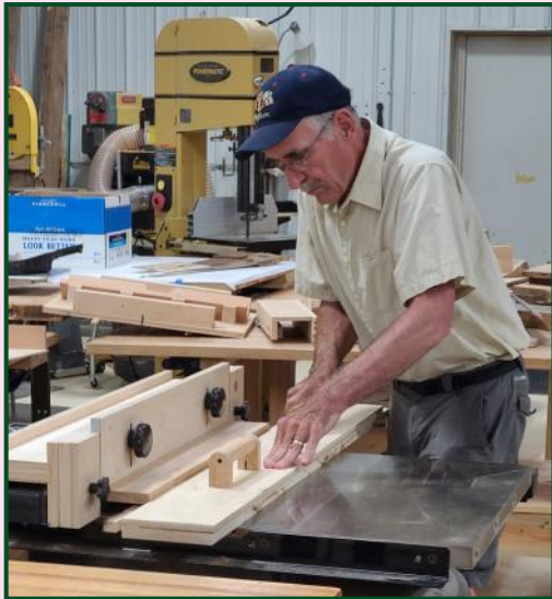
Jim Preusser brought in a spline cutting jig.
