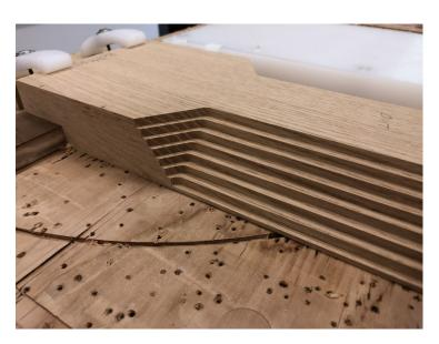
Above & Left: First I when through with a 1/2" dia end mill to rough our the shape. I was left with these neat looking steps.
