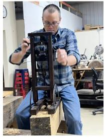
normal shop chisel and the slick used in timber framing. He then demonstrated cutting the mortise using drills to hog out the rough mortise and then cleaning up with chisels. He used three different drills, describing the differences between the drills and the actual bits used with each type of drill.
