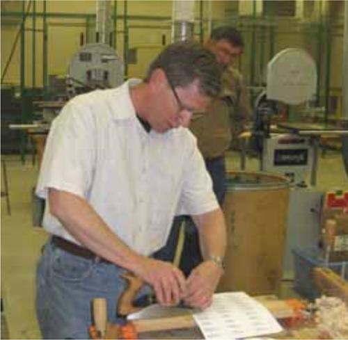
Rollie Johnson picked up where Alex left off by bringing out the big gun. The Lie-Nielsen Large Scraping Plane. It is based on the Stanley #112 which was discontinued in 1944. This is a great tool for smoothing large surfaces such as table tops. Its advantage over the card scraper is with the large flat cast iron base which helps maintain a flat surface. The comfortable handle and knob make scraping enjoyable.
