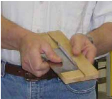
Above: A homemade jig to remove the work hardened steel and put a nice square edge on the card scraper. Its just a piece of scrap wood with a file inserted into a saw kerf.
