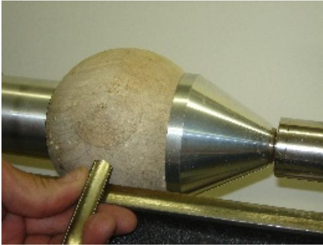
Use a parting tool to separate the ball from the base, catching the ball as its cut free.
