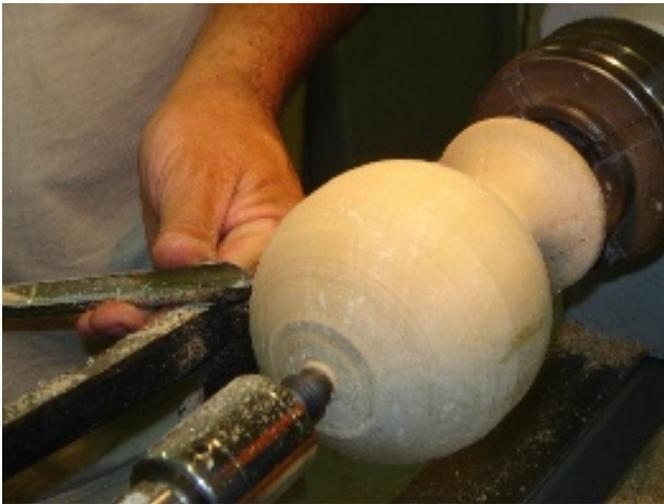
Begin with a piece of wood slightly wider than the desired diameter of the finish ball and 2½" longer. With the wood between centers, use conventional turning techniques to rough out a ball with a tapered base and a tenon (or spigot) to fit your chuck.
