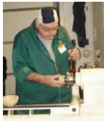
Dick prepares to tap threads in a jam chuck.
