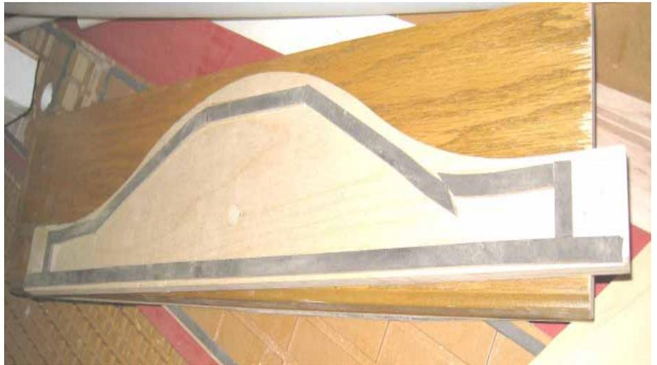
Dave shows us the difference between PVA and Uni-bond 800 glue. PVA remains flexible, while the Uni-bond 800 is very brittle.
