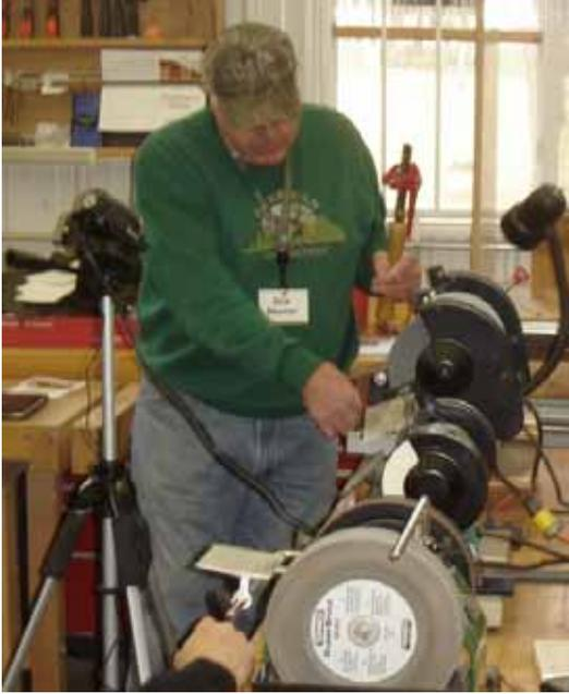
Dick is shown sharpening a turning tool .
